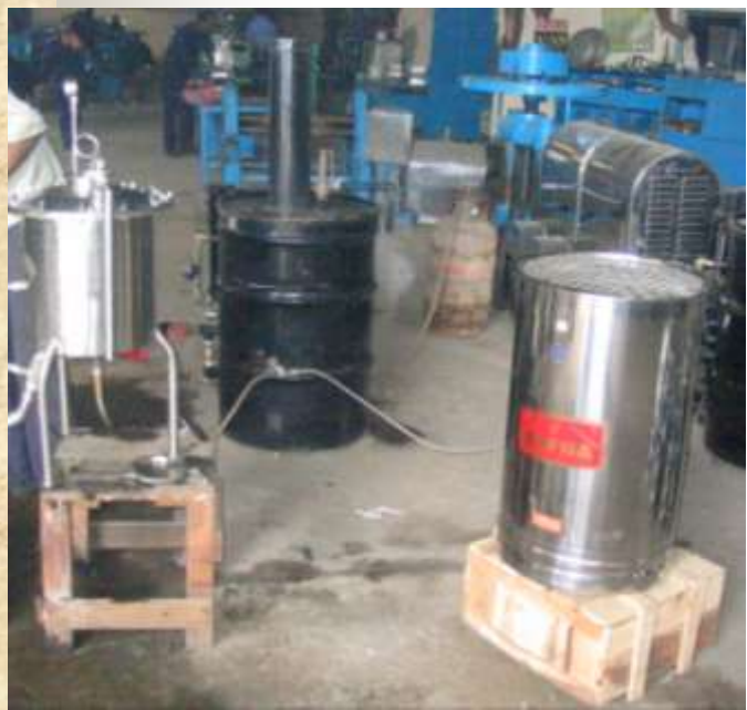
Canning vessel and cooker shown left, both hooked to boiler
